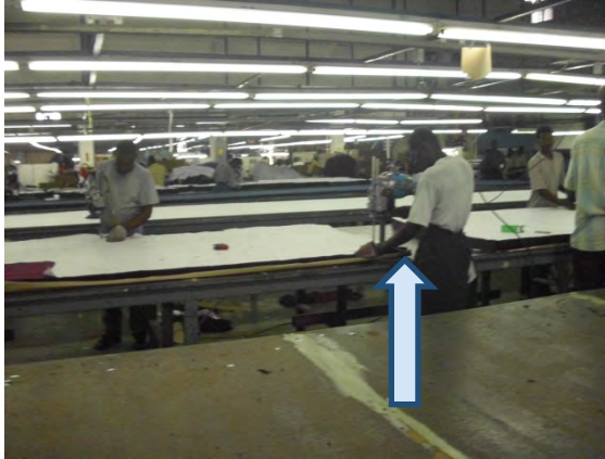
Figure 5. A cutting area in an apparel factory where workers are wearing metal mesh gloves while using blade knife cutters on sheets of fabric. The risk to their hands in the absence of such PPE is clear from the proximity of the hand to the moving blade (arrow).
