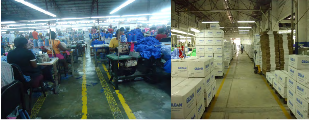
Figure 1. Examples of poor (on the left) and good (on the right) housekeeping and workplace organization, and how these factors may impact means of egress on the factory floor and the ability of workers to evacuate the building. Note on the left how the manufacturing equipment has been allowed to encroach upon the designated egress aisle.
