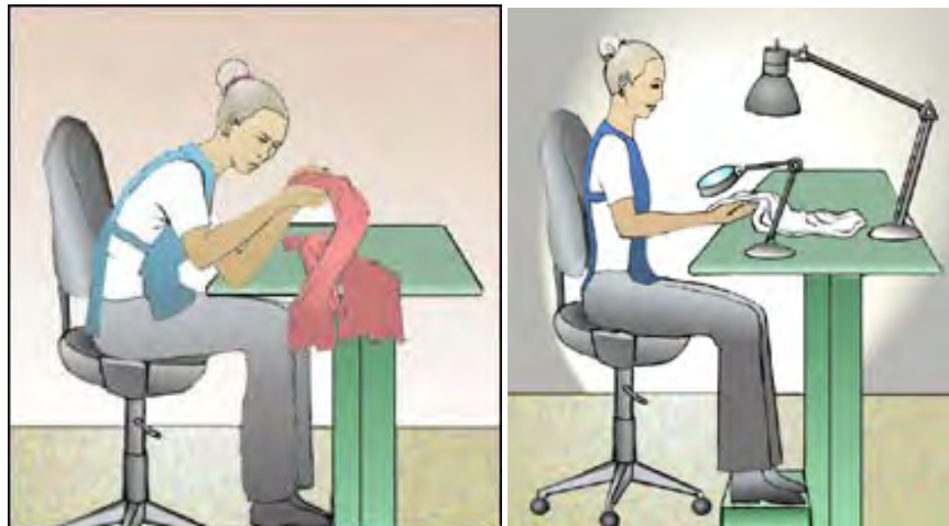
Figure 4. In the illustration on the left, the operator demonstrates poor posture that can lead to strain on the back, neck and shoulders. On the right, the operator achieves good posture with the use of an adjustable chair and a footrest, supporting the upper and lower back and the legs. Task lighting is provided to reduce the tendency to bend in order to inspect the work.
