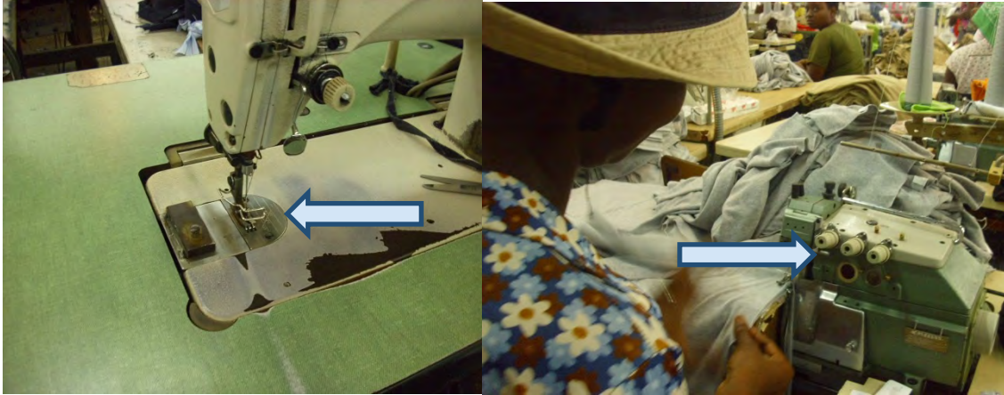
Figure 2. On the left is an example of a needle guard, which protects against puncture injuries, while on the right is an example of an eye guard, which would shield the worker from any flying shards of needle if it should break. Note that the machine on the left is not equipped with an eye guard.
