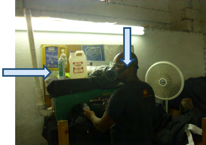
Figure 3. An example of a spot cleaning operation: the respirator is presumably the proper type; that depends upon the specific type of air-purifying cartridges which are provided (vertical arrow). Eye protection is provided, but note that gloves are missing. The ventilation at this work station is questionable: while there appears to be some type of local exhaust ventilation provided via the white pipe (horizontal arrow), the operation of the white fan on the right of the worker would likely disrupt any chance of its effectiveness, and appears to be positioned so that it will blow chemical vapors directly at the worker. Proper chemical selection, location and ventilation could eliminate the need for use of that respirator (imagine wearing it throughout the workday during the summer in Haiti).
