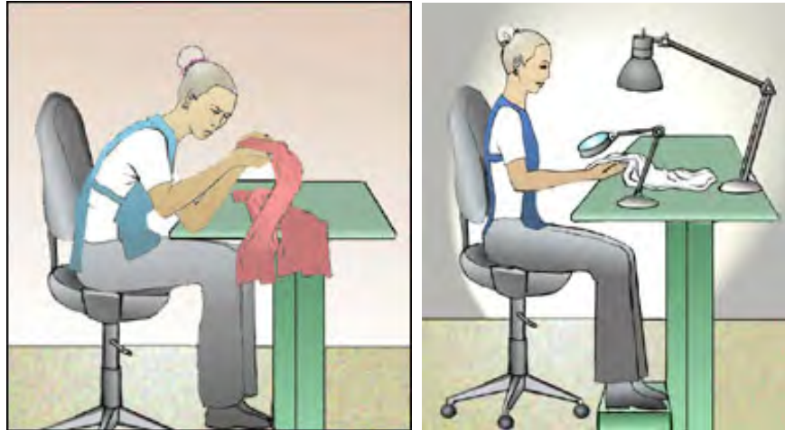
Figure 5. In the illustration on the left, the operator demonstrates poor posture that can lead to strain on the back, neck and shoulders. On the right, the operator achieves good posture with the use of an adjustable chair and a footrest, supporting the upper and lower back and the legs. Task lighting is provided to reduce the tendency to bend in order to inspect the work.
