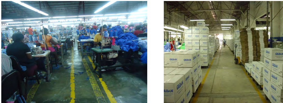
Figure 2. Examples of poor (on the left) and good (on the right) housekeeping and workplace organization, and how these factors may impact means of egress on the factory floor and the ability of workers to evacuate the building. Note on the left how the manufacturing equipment has been allowed to encroach upon the designated egress aisle.
