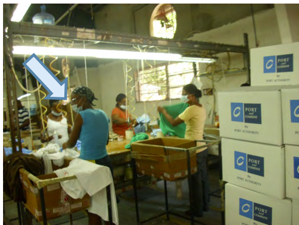
Figure 7. This illustrates the problem which is discussed in the preceding paragraph. The workers at this spot cleaning operation have been provided with loose-fitting dust masks (arrow), which are ineffective against chemical solvent vapors. However, it should also be noted that this location, with windows and overhead exhaust fan, may be preferable for these activities than the location in Figure 4.
