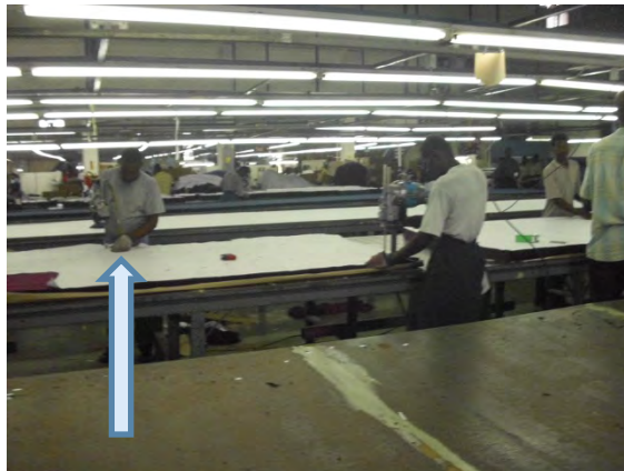
Figure 6. A cutting area in an apparel factory where workers are wearing metal mesh gloves while using blade knife cutters on sheets of fabric. The risk to their hands in the absence of such PPE is clear from the proximity of the hand to the moving blade (arrow).
